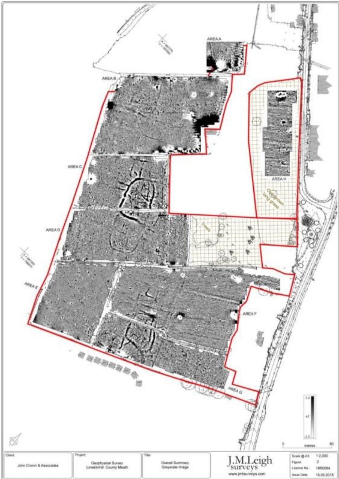
Figure 6: Grayscale image of geophysical survey results
